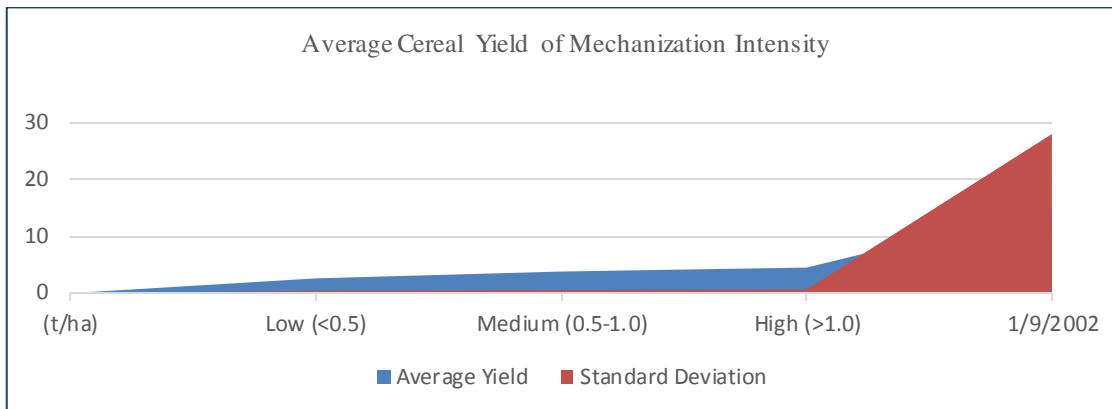
Interpretation: The findings confirm that mechanization significantly enhances productivity, consistent with the Mitscherlich yield response model used in the methodology. However, diminishing returns are observed at the high-intensity level, suggesting that beyond 1.0hp/ha, additional mechanization requires complementary inputs (fertilizers, timely planting) to achieve proportional yield gains.
