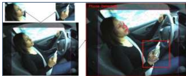
Fig. 1: The bottom left picture displays a camera frame. The top left pictures show the cropped face and hand/phone captures. The right picture shows processed facial landmarks, hand landmarks, and a phone bounding box.
