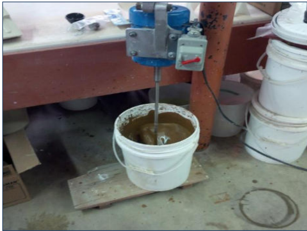
Figure 1. Deflocculation Process in Slip Casting. Propeller-mixing a clay slurry. Source: digitalfire.com
