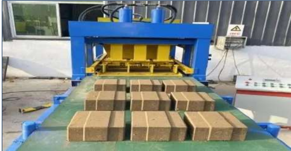
Fig 1.1: Machine-pressed earth block production process in operation(blockmachine1,2024)
